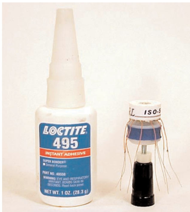
Fig. 5. Shown above is the (printed) circuit board mounting version of the Iso-socket along with the recommended Loctite 495 mounting glue. Note the socket's tinned flying leads.
