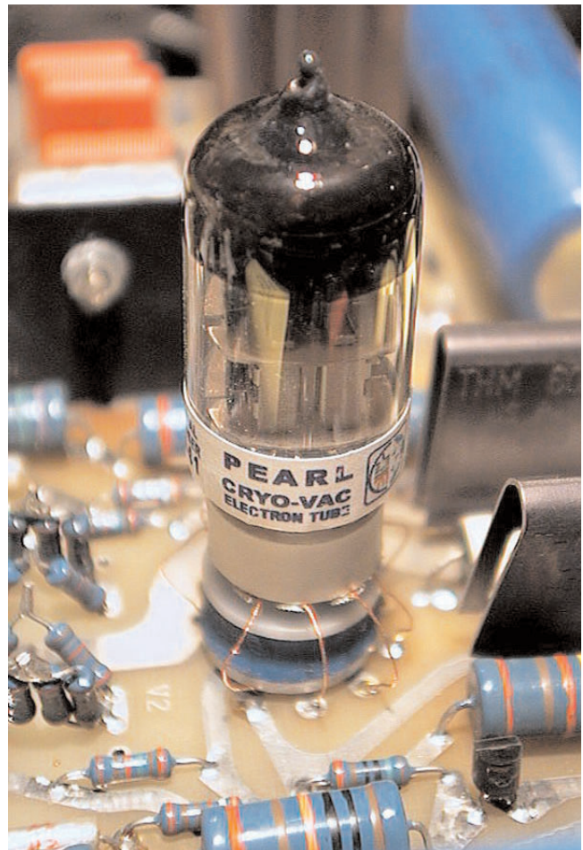
Fig. 7. The installation is here shown completed. Upon completion of soldering be absolutely certain to carefully and thoroughly clean all traces of solder flux from the board. Acetone is recommended for this purpose.
