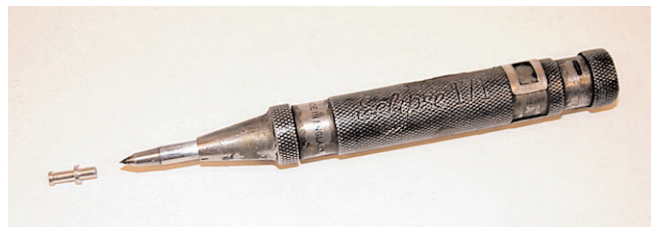
Fig. 8. Shown above are the Keystone, Astoria, NY solder turret and Eclipse, England automatic center punch we use to terminate the flying leads of our Iso-sockets when fitted onto point-to-point wired circuit boards. See Fig. 9 for an enlarged view of the turret
