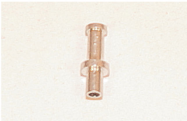
Fig. 9. Shown above is the Keystone 1540-3 turret, suitable for use with a .093" to .100" thick substrates.
